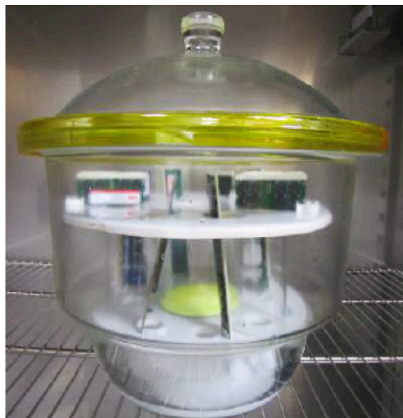
Picture 2: Testing of DRAM modules fitted with anti-sulfuration resistors
